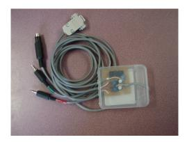
**Background** - This simple interface was developed to capacitive couple audio signals between a radio and PC, to provide a means of adjusting audio levels between a radio and PC and to provide a key-line signal from the PC to a radio. The PC digital software FLDigi was used with the interface but other software could probably be used.
