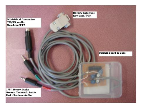
Mini-Din 6 Connector – 6 pin connector that connects to the radio. It connects the Interface board's Audio, Key-line/PTT and Ground signals to the Radio. Verification is recommended, but the pin assignments appear to be the same on ICOM and Kenwood Data connectors and have been tested with both without modification.
