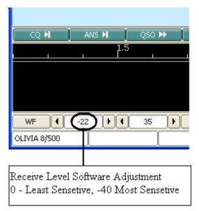
Overdriving the input to the PC will cause the waterfall view to turn RED. No signal will provide a black screen. If needed, adjust the board's potentiometer for a light yellow waterfall with the squelch open and white noise/static is being received, this should allow for a finer adjustment using the GUI. Some adjustment might be needed to suit operating conditions and individual equipment set-up. An oscilloscope can be used to measure the audio level(s).
